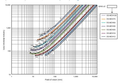
High-speed CMOS camera (standalone) FH-S□02, 2 million-pixel (using 3Z4S-LE VS-MCH series)
