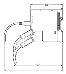
Note: 1. This is the dimension from the back of the unit to the communication cables:
