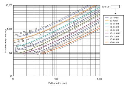
High-speed CMOS camera FH-S $\square$  / High-speed CCD camera FZ-SH $\square$  / Digital CCD camera FZ-S $\square$ , 300,000-pixel (using 3Z4S-LE SV-V series)
