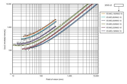
High-speed CMOS camera (standalone) FH-S□04, 4 million-pixel (using 3Z4S-LE VS-MCH series)
