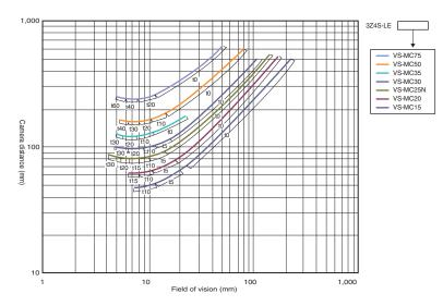
Digital CCD camera FZ-S□2M, 2 million-pixel (using 3Z4S-LE VS-MC series)
