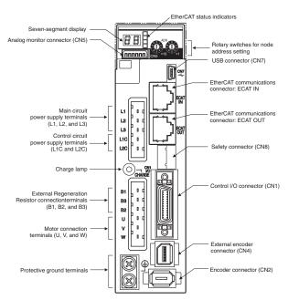
Note: The above picture shows 230 V servo drives models only. The 400 V servo drives have 24 VDC power input terminals for control circuit instead of L1C and L2C terminals.
