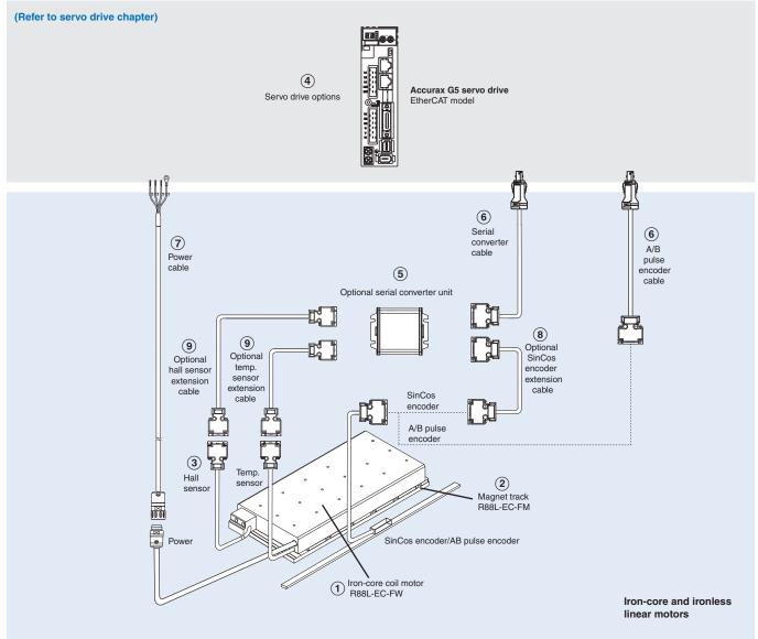
Note: The symbols ①②③... show the recommended sequence to select the linear motor, cables and serial converter for a linear motor system.
