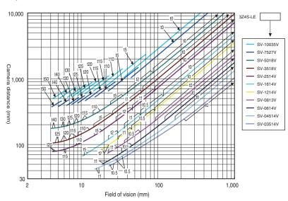
Digital CMOS camera (standalone) FH-S□05R, 5 million-pixel (using 3Z4S-LE SV-H series)
