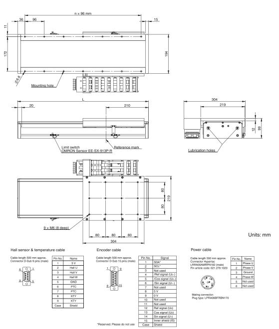
Accurax linear motor axis 279
