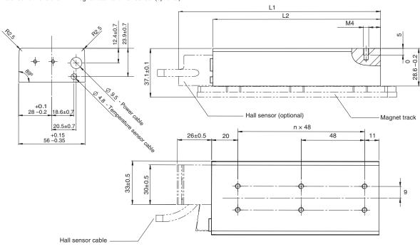
Wiring specifications for motor with connectors
