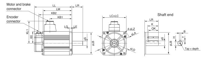
Type 1500 r/min motors (400 V, 7.5 kW)
