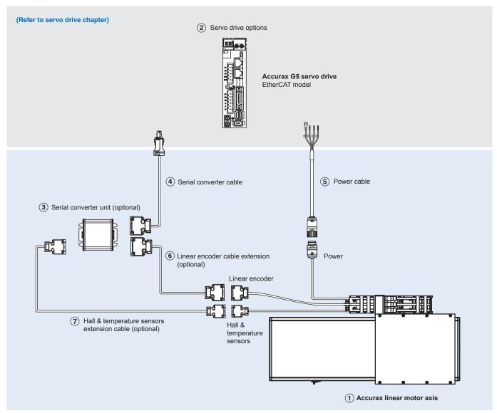
$\textbf{Note:} \ \, \textbf{The symbols 123}... \ \, \textbf{show the recommended sequence to select the servomotor, cables and serial converter for a linear motors system.}$
