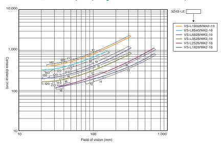
High-speed CMOS camera FH-S□04, 4 million-pixel (using 3Z4S-LE VS-H1 series)
