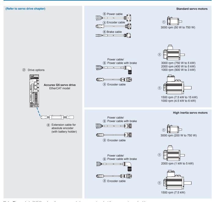
$\textbf{Note:} \ \ \text{The symbols } \ \ \textcircled{123}... \ \ \text{show the recommended sequence to select the servo motor and cables}$
