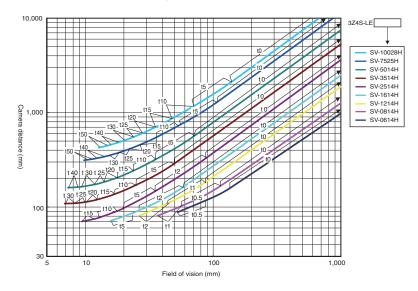
Digital CCD camera FZ-S□2M, 2 million-pixel (using 3Z4S-LE SV-H series)
