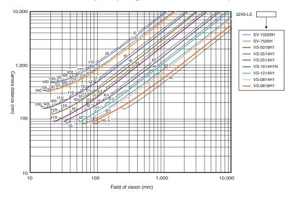
High-speed CMOS camera FH-S□02, 2 million-pixel (using 3Z4S-LE VS-H1 series)
