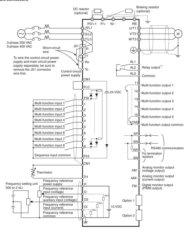
$<sup>^{\</sup>star 1}$   $\;\;$  L is the common reference for analog input and also for the analog output.
