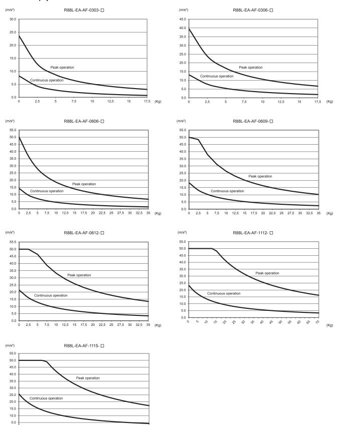
Note: The values on the above curves are calculated based on the below formula and with horizontal orientation:  $Acceleration = (Force-Force_{Friction})/Weigth_{Total}$
