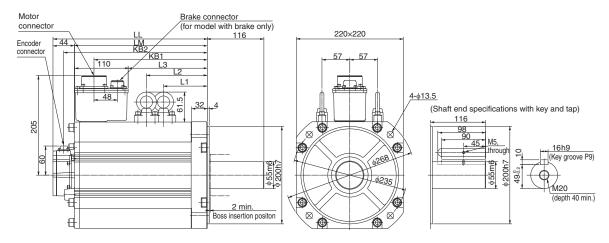
Type 1000 r/min motors (230 V, 900 W/400 V, 900 W to 3 kW)
